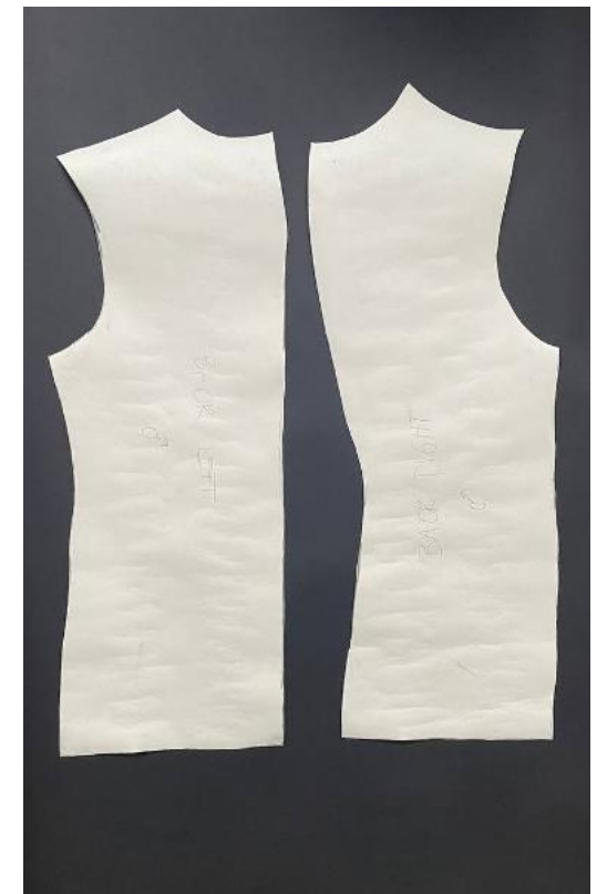
Fig. 73: Sewing pattern, men, back side.
