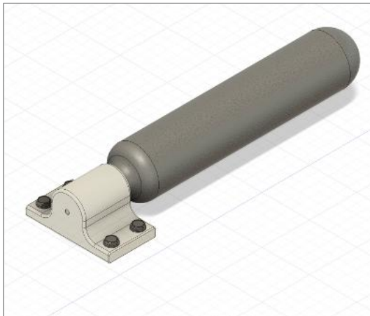
Fig. 55: Carbon dioxide cartridge inside the bracket.
