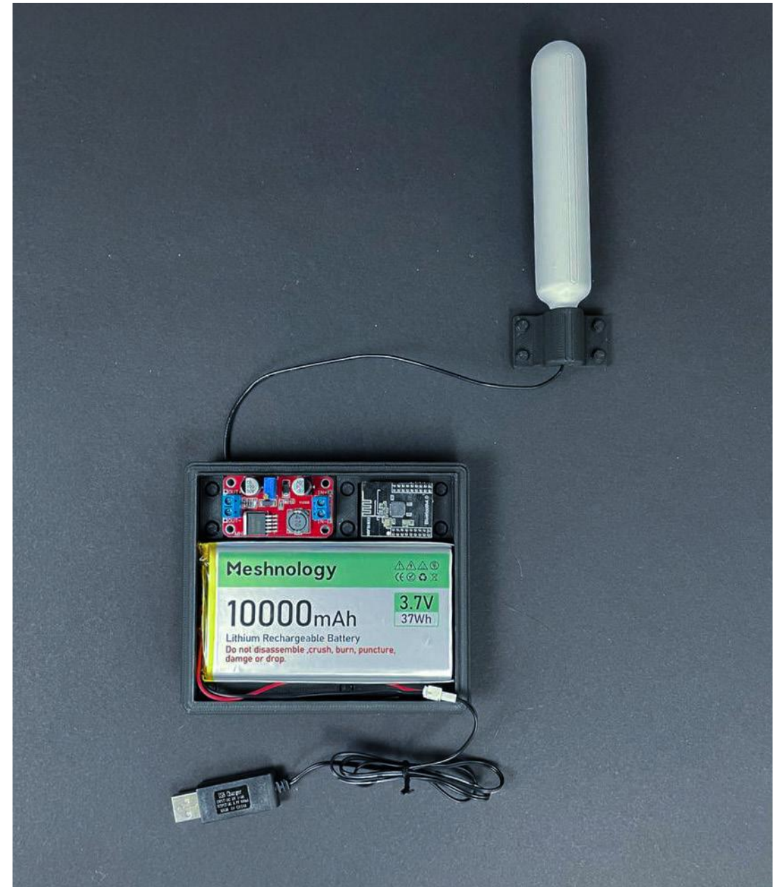
Fig. 109: Carbon dioxide cartridge in bracket, connected to the technical components.
